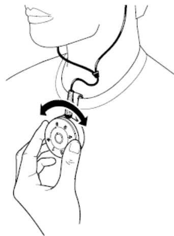
Illustration of how to position the receiver and neck loop (and adjust the volume).
